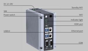
Intel® Core™ i3/i5/i7/Celeron high performance processor, wall-mounted and fanless mini PC
